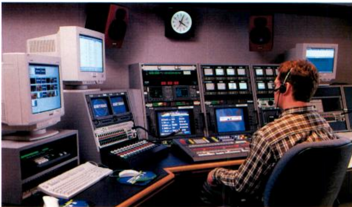
Audio Control Room 9 allows a single operator easy access to critical on-air devices and line-of-sight access to the director.
