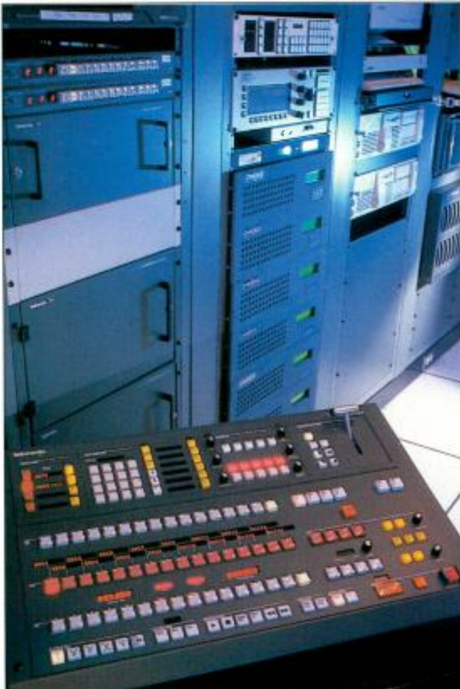
A pair of Grass Valley M-2100 master control systems and OmniBus automation provide the control needed to direct both HD and multichannel operations.
